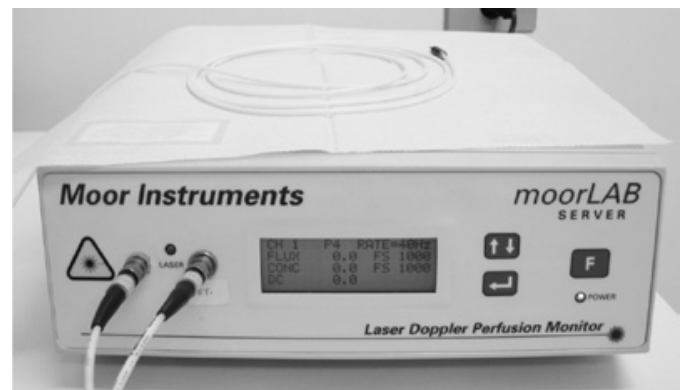
Figura 2. Fluxômetro Laser Doppler da Moor Instruments, moorLAB®.
