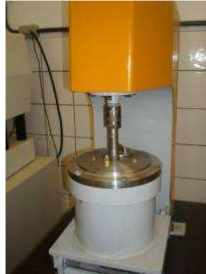
Fig. 2 – Vertical attritor type Mill developed in our laboratory.
