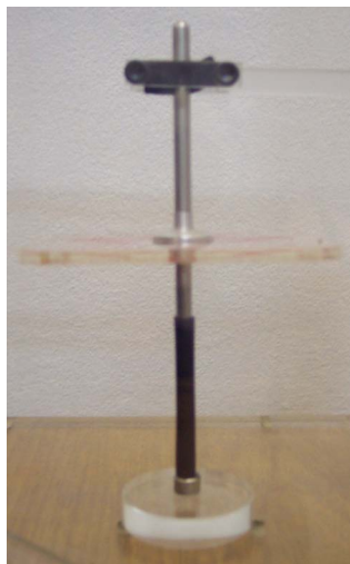
Fig. 2. Experimental set-up for the irradiation of thermoluminescent dosimeters with each clinical applicators.
