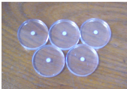
Fig. 7. PMMA supports for \text{CaSO}_4:\text{Dy} pellets of the dosimetric postal system for calibration of ^{90}\text{Sr}+^{90}\text{Y} clinical applicators.
