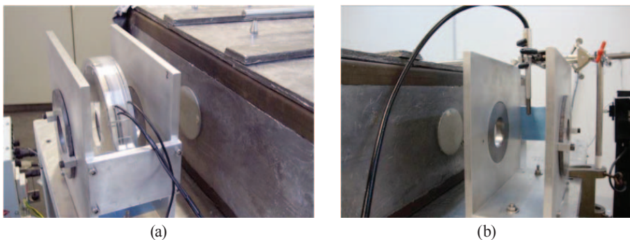
Fig. 2. Ionization chambers positioned in the radiation beam: (a) ring-shaped and transmission chambers (Chamber A); and (b) Farmer-type chamber, in the penumbra region
