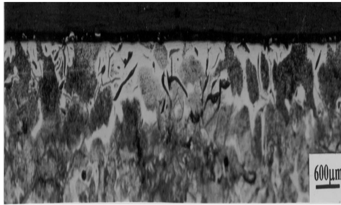
Fig. 7 - OM image of cross-section of gray iron sample with laser track; Condition L5. Nital 4%.
