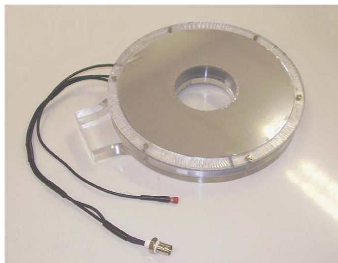
Fig. 2. Photograph of the new monitor chamber.
