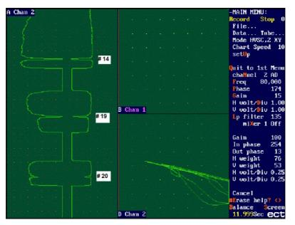
Figure 4. Different amplitude signals obtained for calibration standards numbers 14, 19 and 20.
