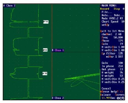
Figure 5. Signals for calibration standards numbers 14, 15 and 16.
