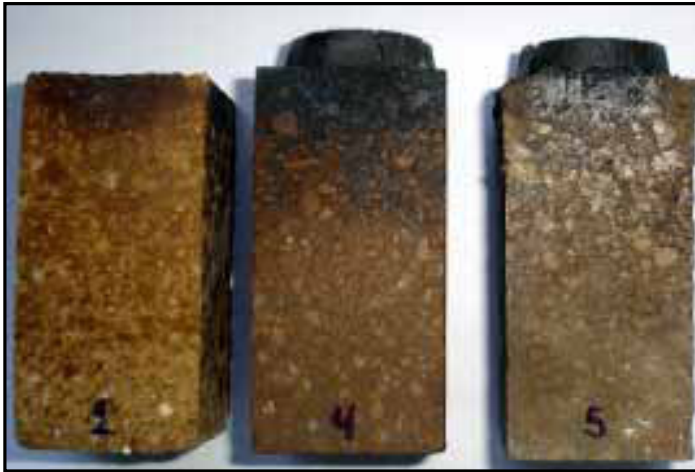
Figure 8. Reaction between Portland cement and MA, MTC 1 and MTC 2 refractories, showing adherence in MTC 1 and MTC 2 compositions.
