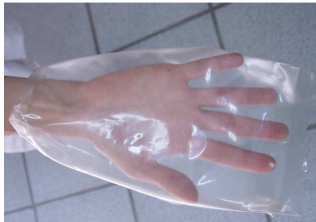
Fig. 1. Illustrative picture of cassava starch edible film (blend of 1.0 g of glycerol; 0.3 g of glutaraldehyde; 0.3 g of polyethylene glycol).
