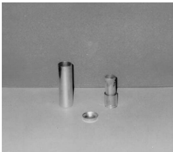
Fig. 1. Irradiation aluminum rabbit, aluminum cap, and a set of Makrofol KG foils containing sample deposits.
