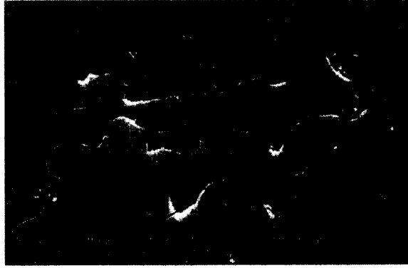
Fig. 3. Secondary electrons micrograph of the grey cast iron cylinder liner, showing graphite type I (homogeneous lamella homogeneously dispersed).
