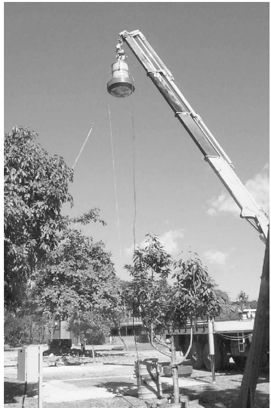
Figure 13. Prototype positioned for the drop test.
