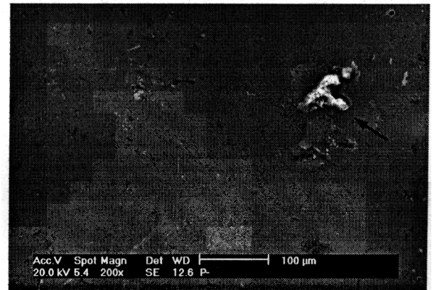
Figure 3 - Localised corrosion at a defect of the coating on St stud. The specimen was immersed for 20 days.
