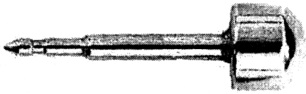
Figure 1 - Macrograph of an ear piercing stud.
