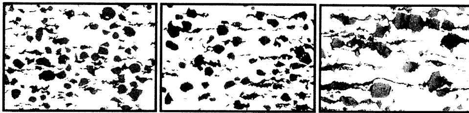
Fig.3 – U 3 O 8 particles after rolling. Fuel plates # : (A)-05/99 - 29% fines; (B)-07/99 - 0% fines (proposed method) and (C)-432 - 0% fines, current method. (550X).
