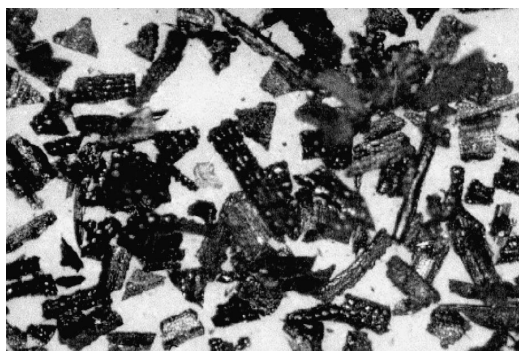
Fig. 2. Optical micrograph showing morphology of rice husk powder.
