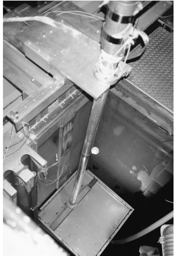
Fig. 8. Photograph of the detection set positioned for measurement at the central point of an irradiated fuel element.
