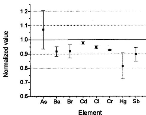
Fig. 1. Normalized values for elemental concentrations obtained in IMEP-10 reference material ( Ratios between of the data obtained at IPEN and IRMM or IRI and the error bars in the figure are uncertainties of IPEN results)
