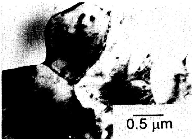
Fig. 6. Transmission electron micrograph for the alloy containing 74.5 at.% Ni, showing bimodal distribution of anti-phase domains: coarse near grain boundaries and fine in the core regions of the grains.
