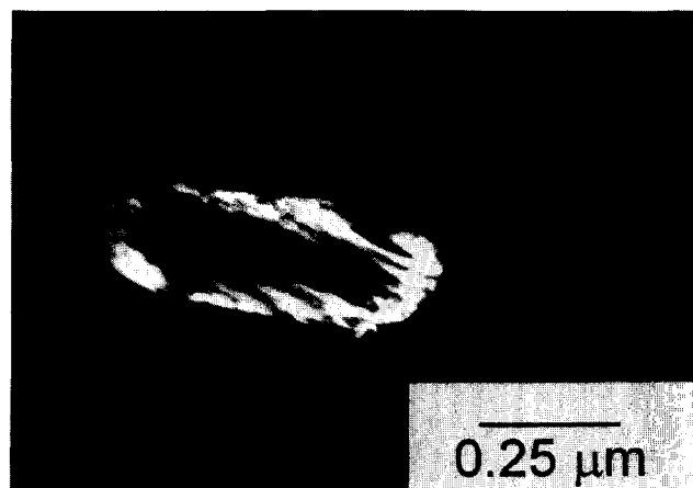
Fig. 5. Transmission electron micrograph (DF) of the martensite phase in the alloy containing 71.9 at.% Ni. These precipitates were observed in the \gamma grains which also had martensite plates of about 0.2 \mu\text{m} width.
