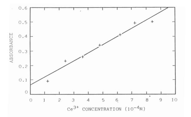
Modified ceric sulphate dosimeter response in function of  $Ce^{3+}$  concentration. Initial  $Ce^{4+}$  concentration:  $1 \times 10^{-4} \text{M}$ .
