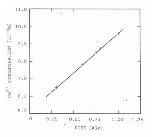
Dose response curve of the modified ceric sulphate dosimeter irradiated with  $^{60}$ Co. Initial Ce $^{4+}$  concentration: 2.99 x  $10^{-4}$ M.
