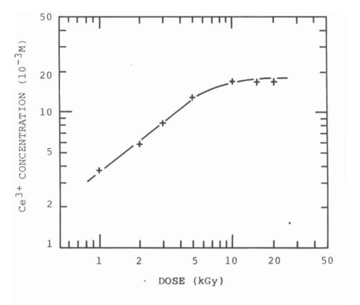
Dose response curve of the modified ceric sulphate dosimeter irradiated with  $^{60}\text{Co.}$  Initial Ce $^{4+}$  concentration: 1.72 x  $10^{-2}\text{M}$ .
