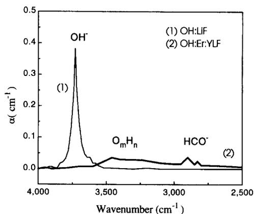
Fig. 2. Absorption spectra of a  $\text{OH}^-$ :LiF crystal (1) compared with  $\text{OH}^-$ : $\text{LiY}_{0.60}\text{Er}_{0.40}\text{F}_4$  (2).
