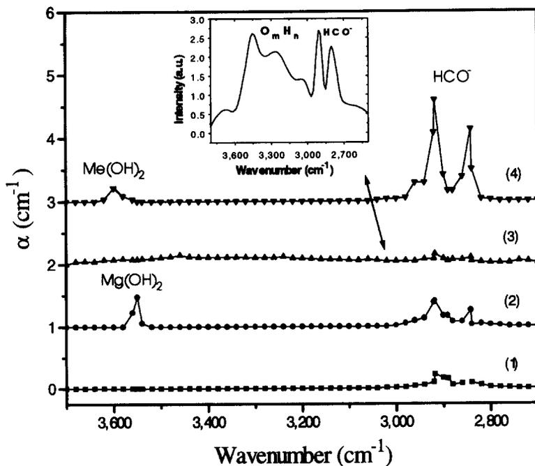
Fig. 1. Absorption spectra of the following crystals: (1)  $\text{LiY}_{0.555}\text{Er}_{0.38}\text{Tm}_{0.06}\text{Ho}_{0.005}\text{F}_4$ , (2)  $\text{Mg}^{2+}:\text{OH}^-:\text{LiY}_{0.60}\text{Er}_{0.40}\text{F}_4$ , (3)  $\text{OH}^-:\text{LiY}_{0.60}\text{Er}_{0.40}\text{F}_4$ . The insert shows in detail the band shape, and (4) commercial YLF.
