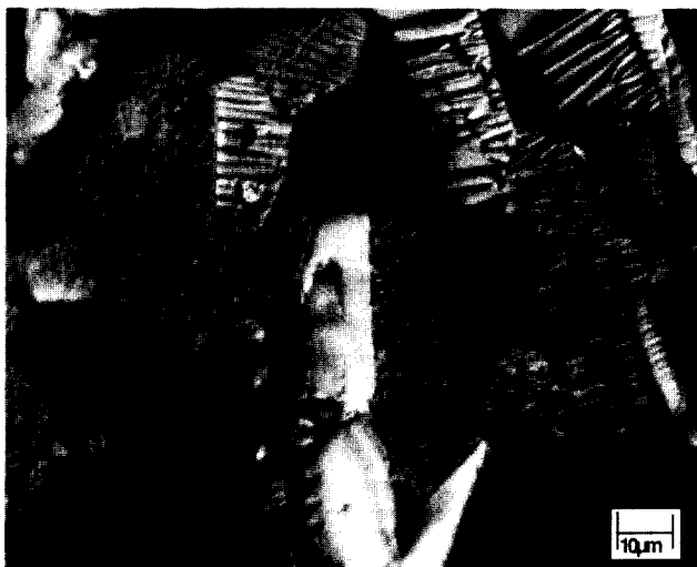
Fig. 6. Ferrofluid picture of the \text{Pr}_{20.5}\text{Fe}_{73.8}\text{Cu}_{2.0}\text{B}_{3.7} alloy, viewed perpendicular to the predominant cooling direction showing that there is rotation of the platelet grains within this section.
