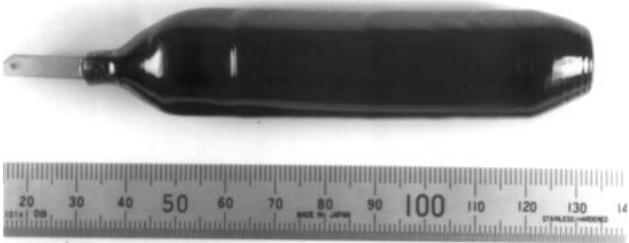
Figure 4 (La, Sr)(Al, Ta)O 3 single crystal grown along the \langle 111 \rangle direction.
