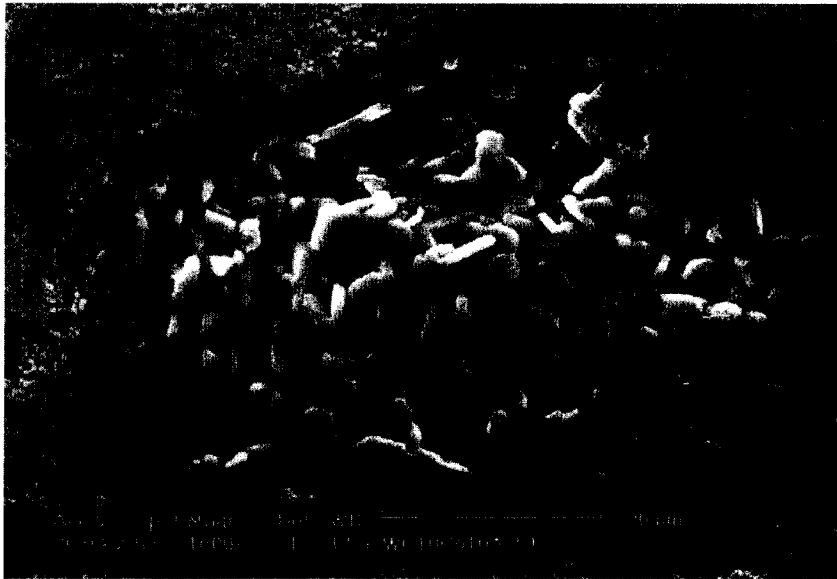
Fig. 3: Microstructure of WC-Co reinforced with 10 wt.% Al 2 O 3 .
