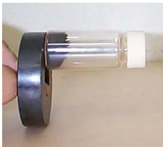
Fig. 6. APTES-magnetite nanoparticles being attracted by a magnet.
