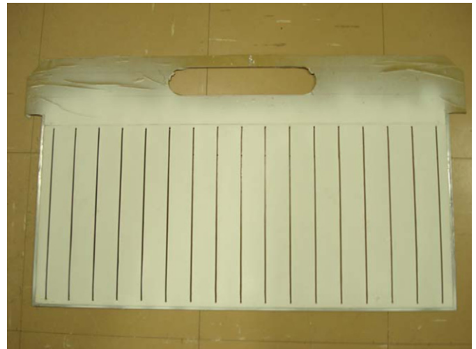
Fig. 10. The slotted absorbent mask used in the 2\theta calibration of the Aurora HRPD.
