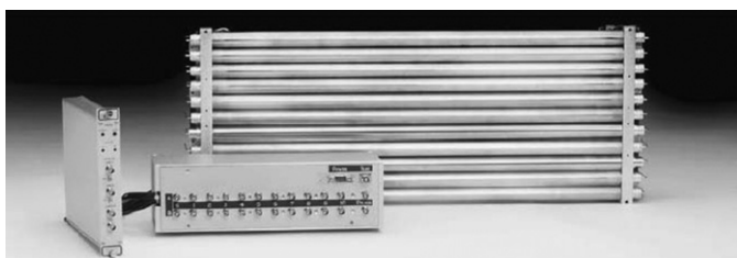
Fig. 2. The neutron PSD array, the junction box and one of the linear PSD signal processing electronics elements (PEMs).
