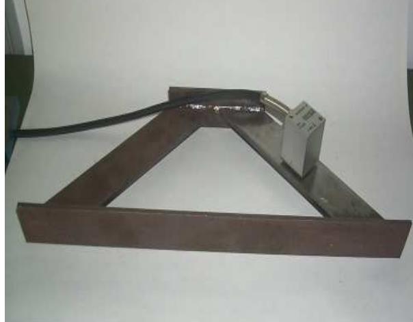
Figure 3. Test specimen and electromagnetic probe.
