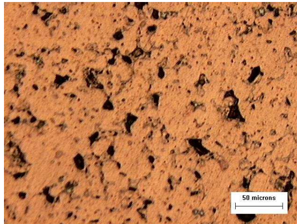
Figure 1 - Optical micrograph of the alloy Cu-0.5%Ni-0.5%Cr, cold compact (1000kPa) and sintered at 780°C for 5,400 s and also homogenized at 500°C for 32,400s.
