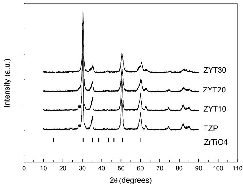
Fig. 1. X-ray diffraction patterns of ceramic samples after sintering at 1350 °C for 01 hour.
