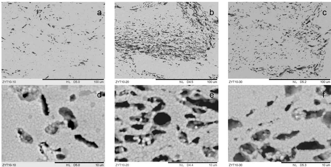
Fig. 3. SEM micrographs of polished and thermally etched surface (a, b and c) and (d, e and f) of samples ZYT10-10, ZYT10-20 and ZYT10-30 with low and high magnification, respectively.
