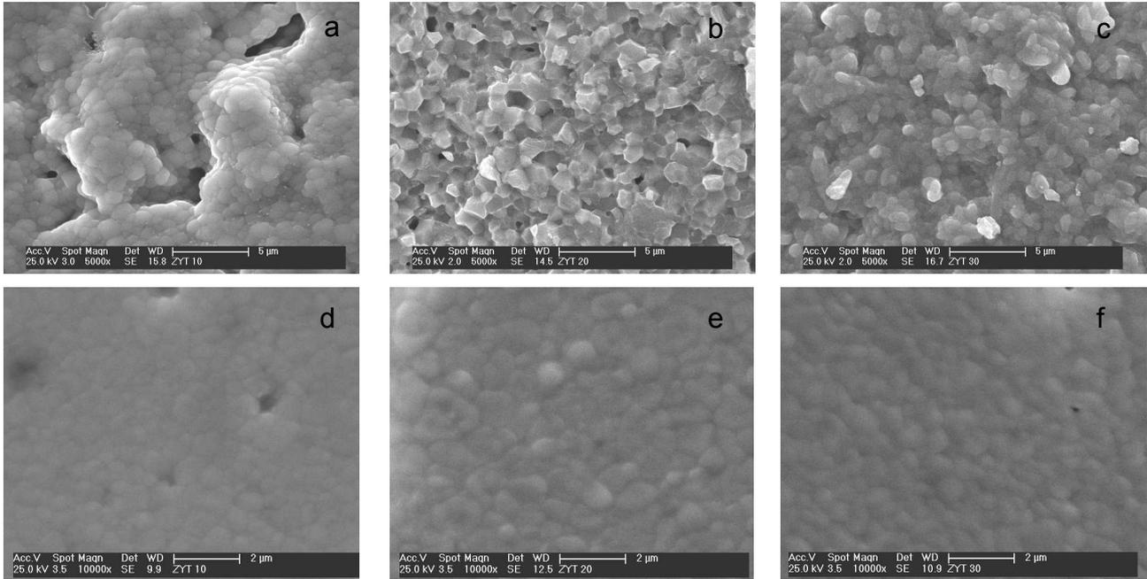
Fig. 2. SEM micrographs of fractured (a, b and c) and polished and thermally etched surface (d, e, and f) of samples ZYT10, ZYT20 and ZYT30, respectively.
