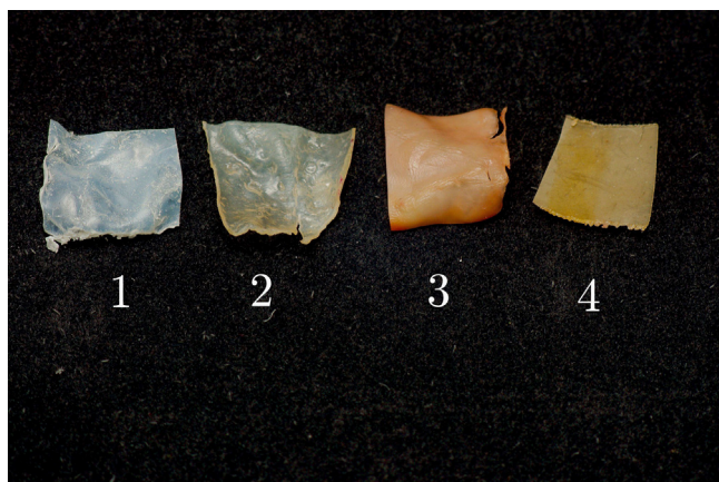
Fig. B2. Physical aspect of the final product. (1) Styrene grafted PP-1, with high yield of grafting (not chemically modified). (2) Chemically modified PP-1 (low yield – first step of modification). (3) Chemically modified PP-1 (high yields – first step of modification and grafting). (4) Chemically modified PP-2 (high yield for the first modification and low yield of grafting).
